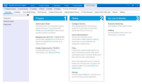
Step 4 Select Deployment from the left-hand pane to jump to the page Device Administration Deployment. Since this ISE is standalone, select either [⊙ All Policy Service Nodes ] or [⊙ Specific Nodes ] and select ✓ your ISE node (e.g.:ise-1.demo.local), under Activate ISE Nodes for Device Administration.
