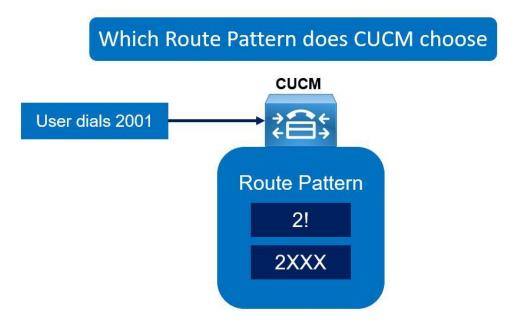
Route Pattern the **2!** pattern matches an infinite number of digits because the pattern matches a variable number of digits but for the purposes of closest-match routing, digit
