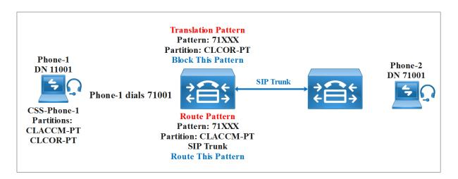
The **Phone-2** will ring because when we have equals match in this case a Translation Pattern and a Route Pattern then CUCM uses higher Partition in CSS (the Partition listed first). In this case **CLACCM-PT** is higher than **CLCOR-PT** so it will match the Route Pattern and will routes the call. So the **Phone-2** will ring because the RP is listed first in the partitions list.
