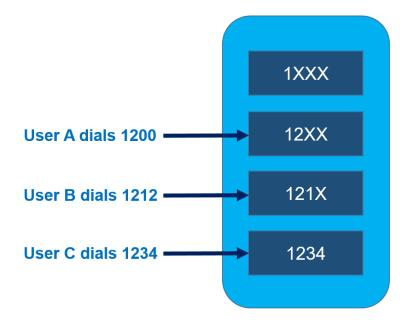
When User A dials the string **1200**, Cisco Unified Communications Manager compares it to the patterns in its call-routing table. In this case, there are two potentially matching patterns: **1XXX** and **12XX**. Both of these patterns match the dialed string, but 1XXX matches a total of 1000 strings (from **1000** to **1999**), whereas **12XX** matches only 100 strings (from **1200** to **1299**).
