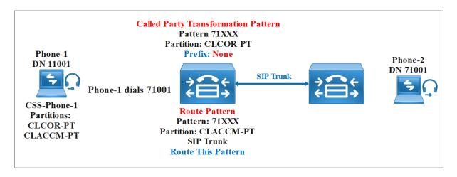
The **Phone-2** will not ring. The Called Transformation Pattern is applied after the routepattern decision and after the Gateway or SIP Trunk Selection. Here what happen, the **Phone-1** CSS has access to the Called Transformation Pattern Partition, this Partition is listed first, the result is that there is a blackhole. and the call will not be routed.
