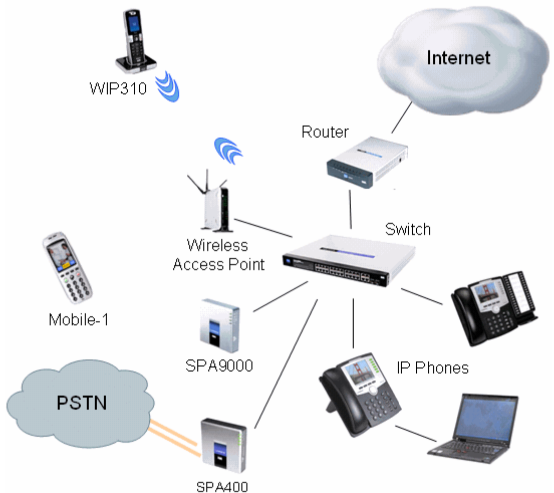
Figure 1 Network Overview: SPA9000 Voice System with Wireless Access Point
