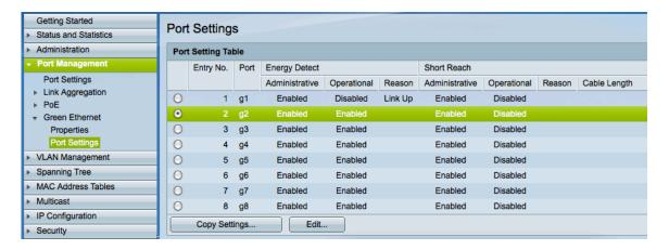
**STEP 9.** Check the desired port to configure, and click Edit at the bottom of the page. A pop-up block will appear where you will be able to set the Energy detection capabilities of that port
