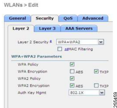
Figure 8-28 Incompatible WPA and WPA2 Security Encryption Settings for OEAP 600 Series.
